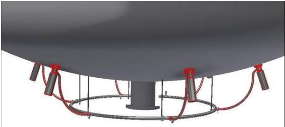
Figure 1 – Schematic Presentation of the bottom of the kettle equipped with an external ring system.
