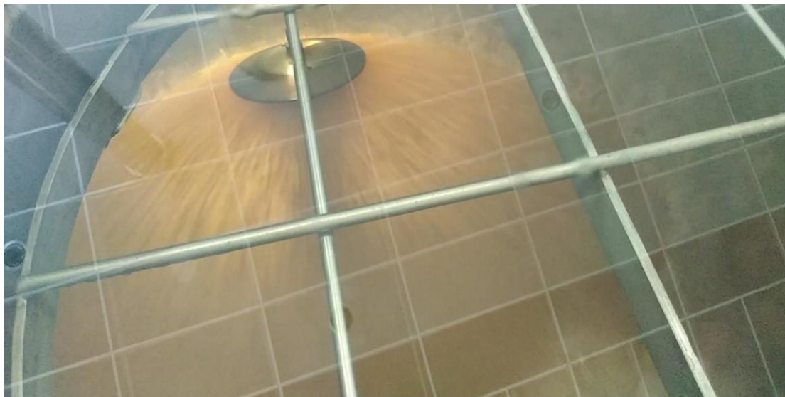
Figure 2 -Wort breaking down the foam due to deflector effect inside the kettle
